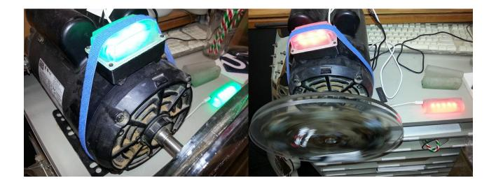
When the motor is not spinning, the light on the SeeSaw will be green.
